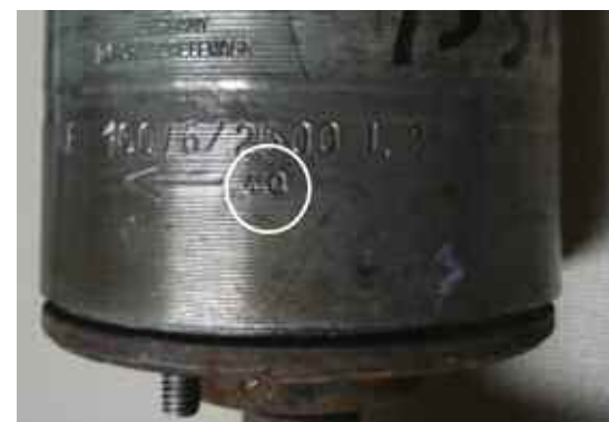
From top: Bosch coil date code. Yes, they are there under the paint. 1Q date code represents January 1959. Photo by John Hawkins. 7S date code (July '61) on a Bosch distributor. You really have to clean to find these stamps, but they are normally in the location shown in this shot. Photo by Chris Ralston. Steve Proctor provided this shot of a Bosch Generator. Date code 4 Q, from April 1959.
