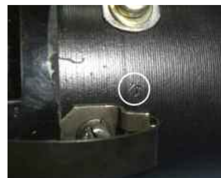
From top: Bosch coil date code. Yes, they are there under the paint. 1Q date code represents January 1959. Photo by John Hawkins. 7S date code (July '61) on a Bosch distributor. You really have to clean to find these stamps, but they are normally in the location shown in this shot. Photo by Chris Ralston. Steve Proctor provided this shot of a Bosch Generator. Date code 4 Q, from April 1959.
