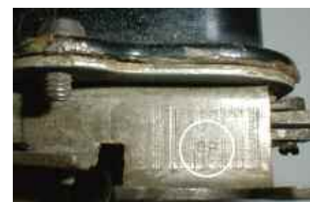
From top: Bosch condenser with date code 2P, (February 1958). Photo by Curt Crowell. Bosch Windshield Wiper motor with a date stamp of 10, indicating Oct. '64 production. Photo by Curt Crowell. 8P date code (August 1958) on Bosch regulator. Photo by John Chatley. Bosch Horn picture below, Julian Hardy. Date is on the flange through which the screws go. The 3Q stamp means production in March, 1959.
